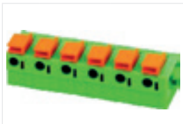
DG142R-7.62 CE 450V/15A 0.2-1.5mm 2 UL 300V/10A 22-16AWG Pola/Poles 1P-XXP
