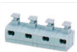
DG235T-10.0 CE 250V/10A 2X-0.75mm 2 UL 300V/5A 20-18AWG Pola/Poles 1P-XXP
