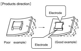
Products shall be located in the sideways direction (Length:a<br/>b) to the mechanical stress.
