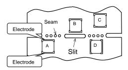
\*1 A > D is valid when stress is added vertically to the perforation as with Hand Separation.
