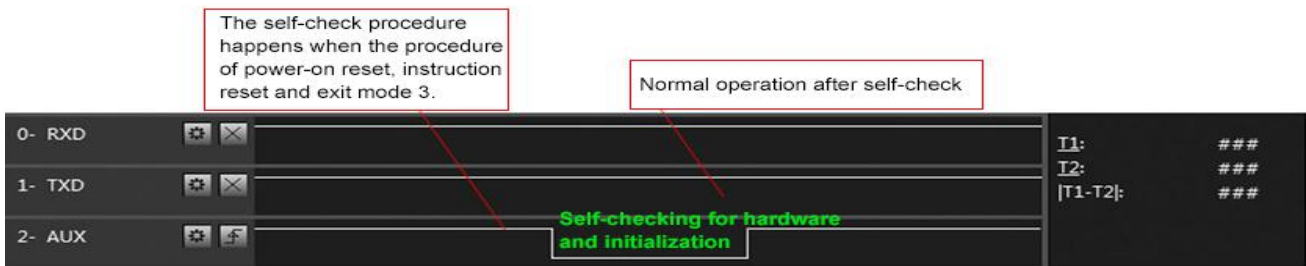
Timing Sequence Diagram of AUX when self-check
