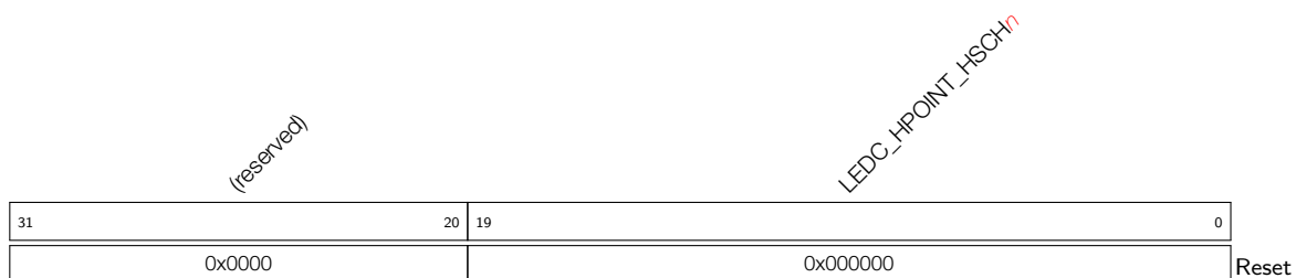
Register 14.2: LEDC_HSCH n _HPOINT_REG ( n : 0-7) (0x20+0x10* n )
