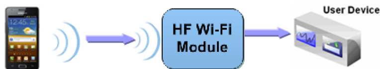
Figure 40. Wireless Control Application
