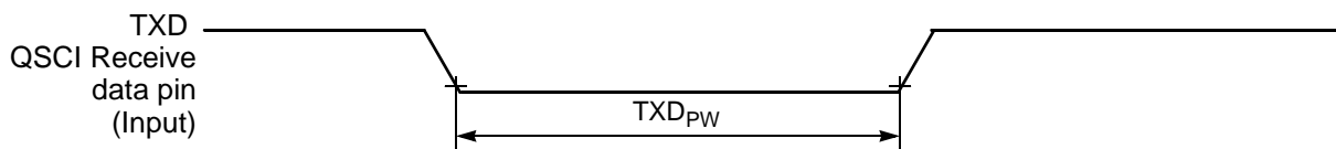
Figure 10-13 TXD Pulse Width
