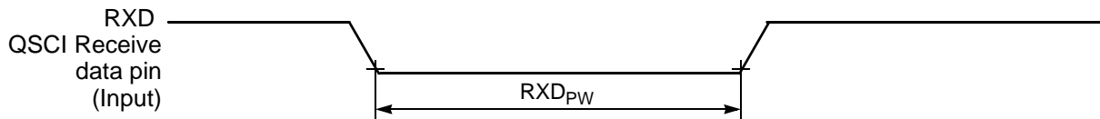
Figure 10-12 RXD Pulse Width
