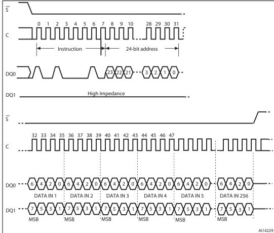
Figure 20. Dual Input Fast Program (DIFP) instruction sequence
