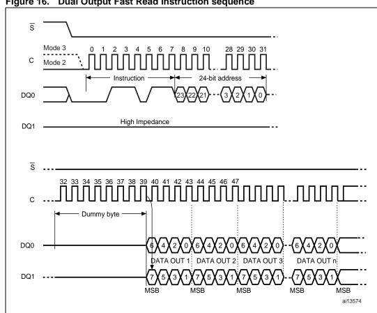
Figure 16. Dual Output Fast Read instruction sequence
