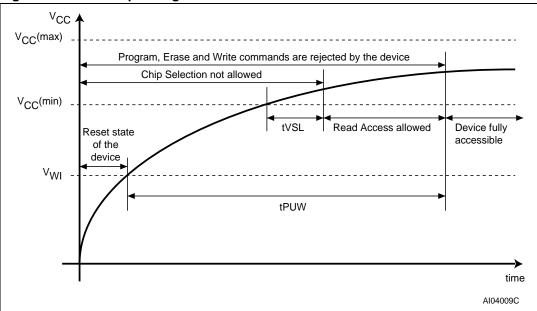
Table 11. Power-up timing and  $V_{WI}$  threshold
