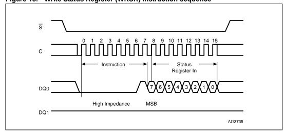
Figure 13. Write Status Register (WRSR) instruction sequence
