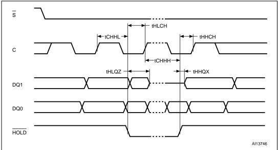
Figure 34. Output timing
