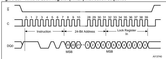
Figure 23. Write to Lock Register (WRLR) instruction sequence
