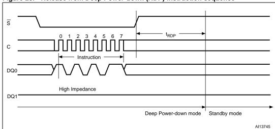
Figure 28. Release from Deep Power-down (RDP) instruction sequence
