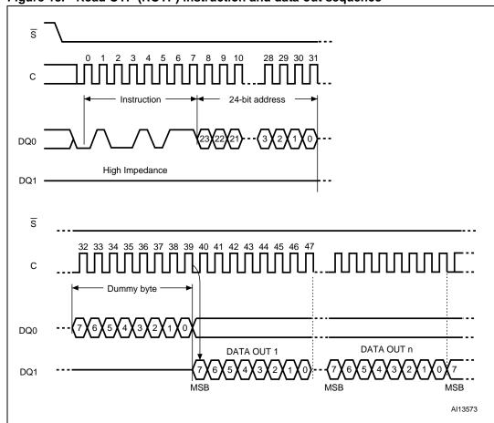
Figure 18. Read OTP (ROTP) instruction and data-out sequence
