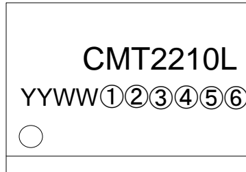
Figure 14. CMT2210L Top Marking
