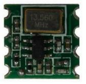
supply. CYT60 has all the characteristics for FCC/CE certification. CYT60 can achieve wireless data signal input to wireless signal output. Users can easily achieve the development of wireless products by adding a simple data decoding circuit
