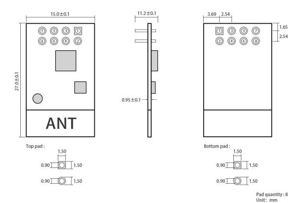
Pin No. Pin item Pin direction Pin application **GND** Ground 1 2 VCC Power supply must be  $20. \sim 3.6 V$ -3 CE Input Chip Enable CSN SPI Chip select 4 Input 5 SCK Input SPI clock MOSI 6 Input SPI master output slave input 7 MISO Output SPI master input slave output 8 IRQ Output Interrupt request.
