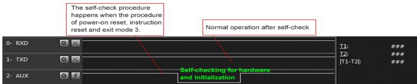
Timing Sequence Diagram of AUX when self-check
