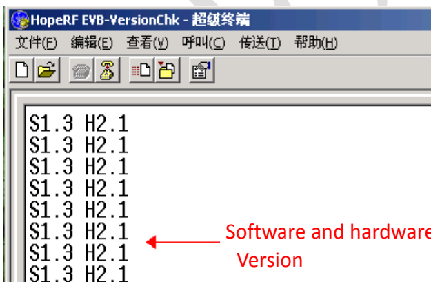
Figure 8 back of the UART interface and the corresponding display effect
