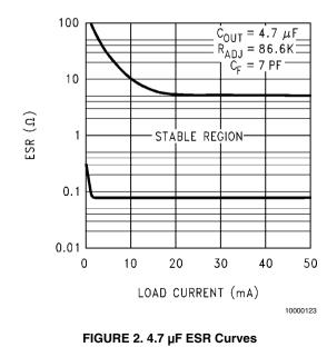
**IMPORTANT:** The output capacitor must maintain its ESR in the stable region *over the full operating temperature range* to assure stability. Also, capacitor tolerance and variation with temperature must be considered to assure the minimum amount of capacitance is provided at all times.
