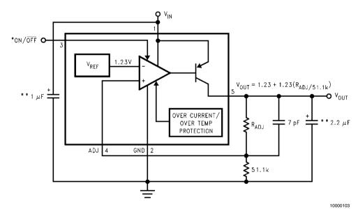
\*ON/OFF INPUT MUST BE ACTIVELY TERMINATED. TIE TO V<sub>IN</sub> IF THIS FUNCTION IS NOT TO BE USED. \*\*MINIMUM CAPACITANCE IS SHOWN TO ENSURE STABILITY OVER FULL LOAD CURRENT RANGE (SEE APPLICATION HINTS).
