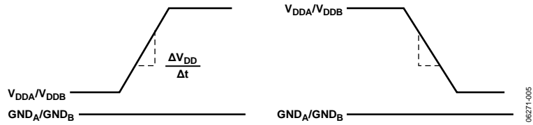
Figure 14. Transient Immunity Waveforms—Output Supplies
