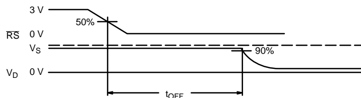
FIGURE 3. t_{OFF} from \overline{RS}
