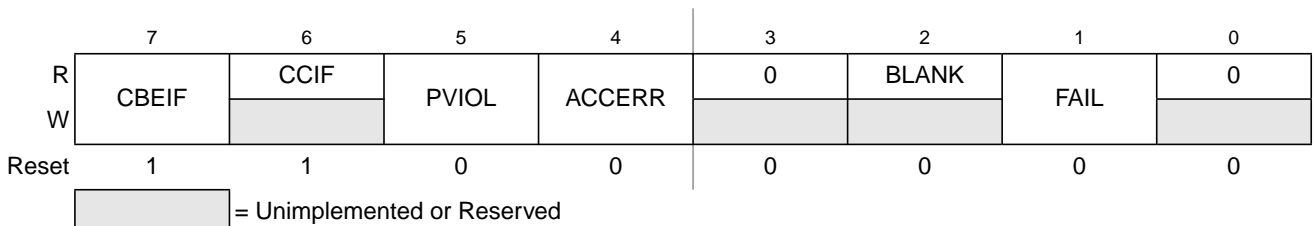
Figure 25-10. EEPROM Status Register (ESTAT — Special Mode)
