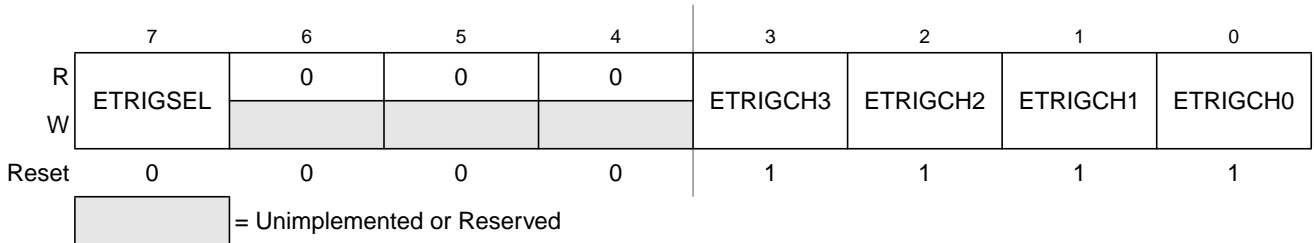
Figure 4-4. ATD Control Register 1 (ATDCTL1)
