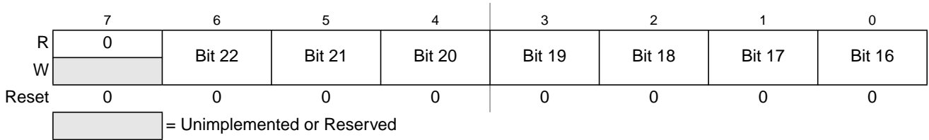
Figure 20-15. Debug Comparator Address High Register (DBGXAH)
