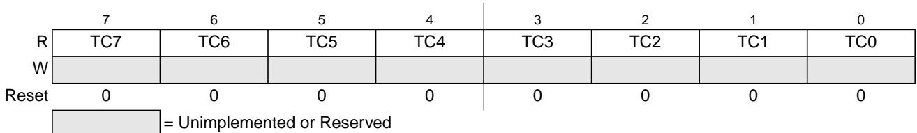
Figure 7-58. Timer Input Capture Holding Register 0 Low (TC0L)
