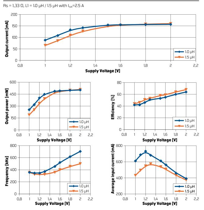
The peak input current is approximately twice the average input current. At some conditions this current is close to the SW current maximum rating. The allowed ambient temperature range is restricted by the maximum junction temperature rating!
