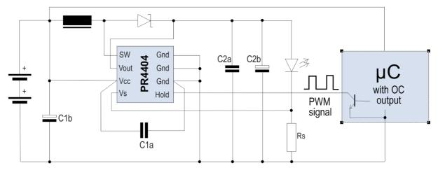
Mind that no voltage must be applied at the Hold pin, but it must only be pulled down to Gnd. Only an open collector or open drain output must be connected to Hold! Due to the remaining quiescent current this feature is not recommended for soft-switching battery-operated lamps on and off.
