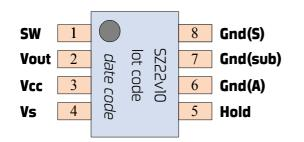
**Pin No Pin Name Pin Function Description** SW 1 driver output 2 Vout output voltage, rectified З Vcc battery supply input 4 Vs LED cathode / current sense resistor 5 Hold shutdown 6 Gnd (A) ground (analog)\* 7 Gnd (sub) ground (substrate)\* 8 Gnd (S) ground (power)\*
