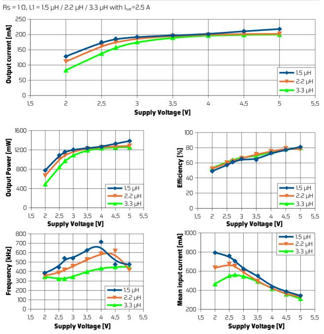
As PR4404 is a boost converter, input voltages higher than the LED forward voltage require two or three LEDs in series at the output. With two LEDs in series, a stable output current of 200 mA, or an output power of 1.2 W, can be achieved in the voltage range between 3.5 V and 5 V, which is interesting for three battery cell applications. Operation with a 2.2  $\mu$ H yields optimum results with best margins.High input currents that occur at low input voltages can thermally overload the IC.
