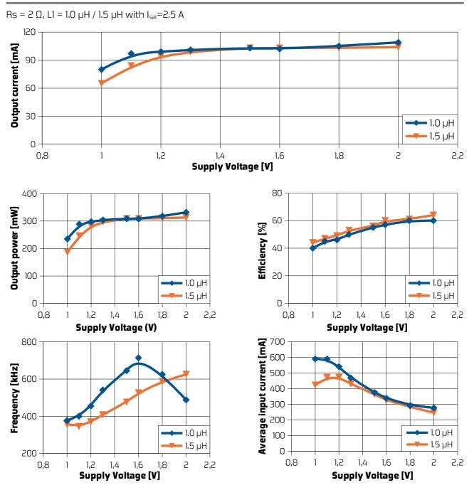
For best operation at supply voltages between 1.0 V and 1.6 V the 1.0  $\mu$ H inductance is the best choice, while at higher voltages 1.5  $\mu$ H are recommended. Generally, the peak input current is approximately twice the average input current.
