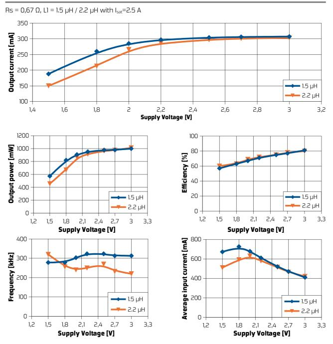
The peak input current is about twice the average input current. At some conditions this current is close to the SW current maximum rating. The allowed ambient temperature range is restricted by the maximum junction temperature rating!
