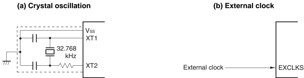
Figure 5-24. Example of External Circuit of XT1 Oscillator
