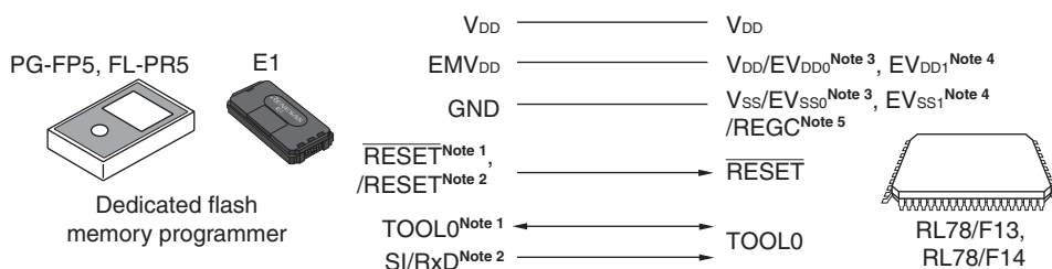
Figure 30-2. Communication with Dedicated Flash Memory Programmer
