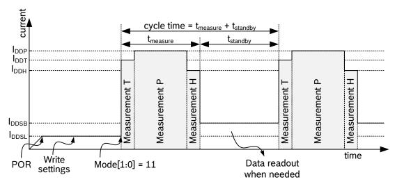
Figure 5: Normal mode timing diagram
