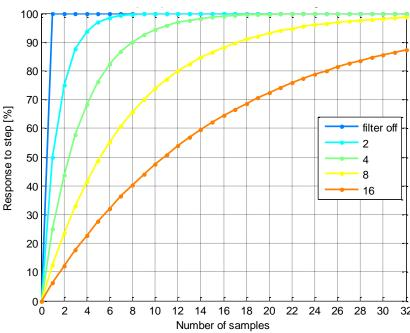
Figure 7: Step response at different IIR filter settings
