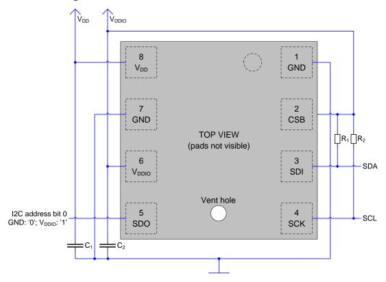
Figure 17: I2C connection diagram
