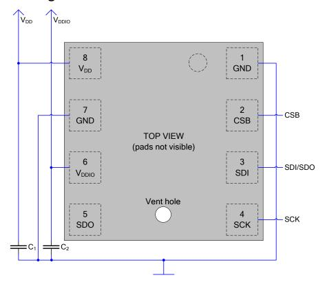
Figure 19: 3-wire SPI connection diagram
