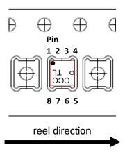
Figure 24: Orientation within tape
