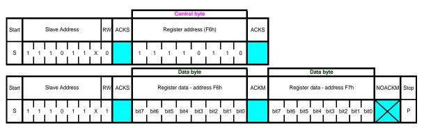
Figure 10: I2C multiple byte read
