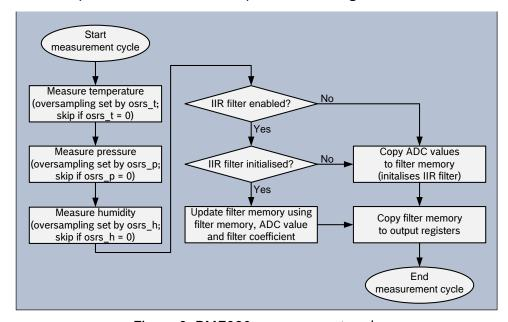
Figure 6: BME280 measurement cycle
