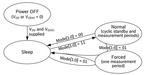
Figure 3: Sensor mode transition diagram
