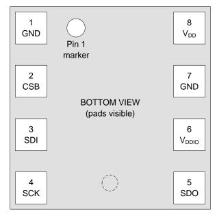
Figure 16: Pin-out top and bottom view
