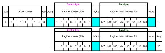
Figure 9: I2C multiple byte write (not auto-incremented)
