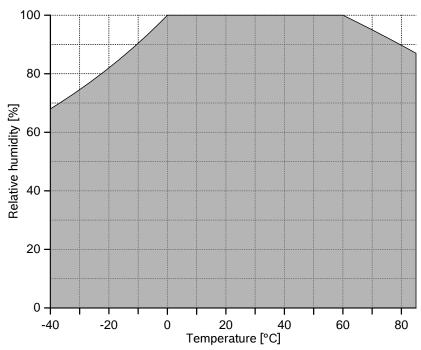
Figure 1: humidity sensor operating range
