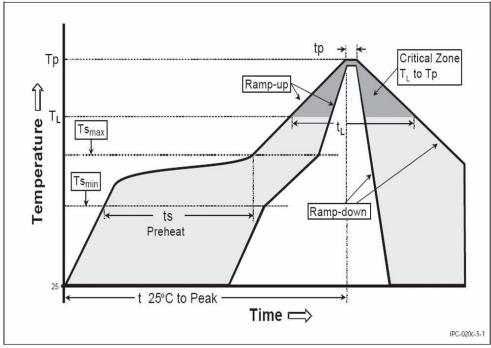
Figure 22: Soldering profile
