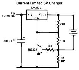
\*Sets peak current,  $I_{PEAK} = 0.6V/R1$ \*\*1000µF is recommended to filter out any input transients.
