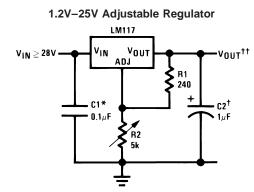
Full output current not available at high input-output voltages \*Needed if device is more than 6 inches from filter capacitors.
