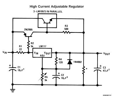
‡Optional — improves ripple rejection †Solid tantalum \*Minimum load current = 30 mA
