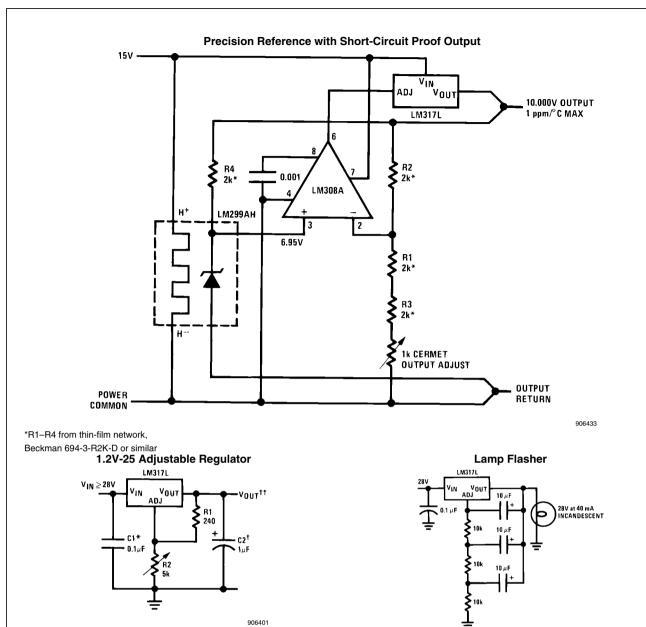
Full output current not available at high input-output voltages †Optional—improves transient response
