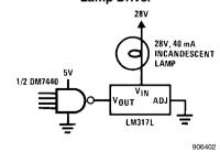
Output rate—4 flashes per second at 10% duty cycle
