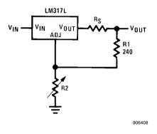
FIGURE 2. Regulator with Line Resistance in Output Lead
