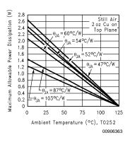
FIGURE 10. Maximum Allowable Power Dissipation vs. Ambient Temperature for TO-252
