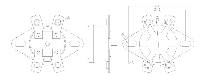
2.2 Terminal Strength: Terminals can bear tensile force of 48N and thrust
