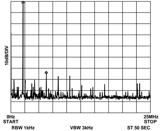
Figure 12.  $f_{MCLK} = 50$  MHz,  $f_{OUT} = 2.1$  MHz. Frequency Word = ACO8312
