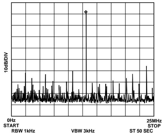
Figure 17.  $f_{MCLK} = 50$  MHz,  $f_{OUT} = 13.1$  MHz. Frequency Word = 43126E98
