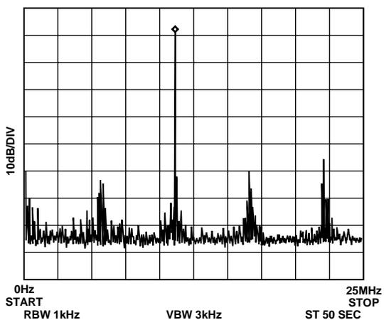
Figure 16.  $f_{MCLK} = 50$  MHz,  $f_{OUT} = 11.1$  MHz. Frequency Word = 38D4FDF4
