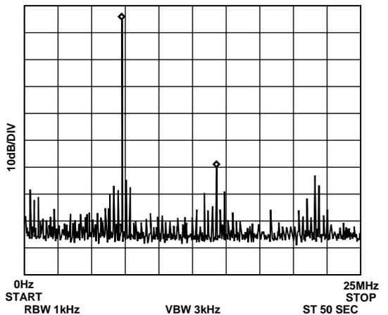
Figure 14.  $f_{MCLK} = 50$  MHz,  $f_{OUT} = 7.1$  MHz. Frequency Word = 245AICAC
