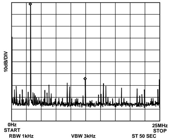
Figure 13.  $f_{MCLK} = 50$  MHz,  $f_{OUT} = 3.1$  MHz. Frequency Word = FDF3B64
