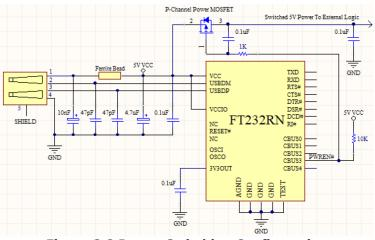
Figure 2.8 Power Switching Configuration
