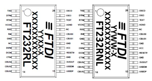
Figure 2.1 FT232RL and FT232RNL Pin Out
