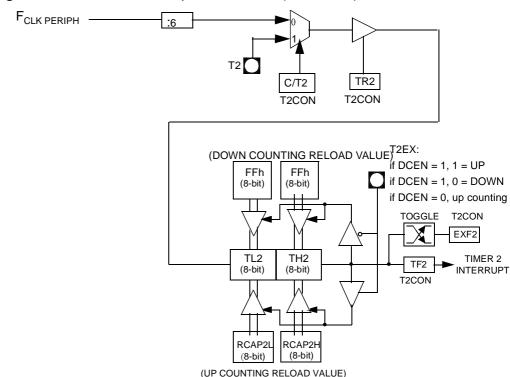
Figure 9. Auto-Reload Mode Up/Down Counter (DCEN = 1)
