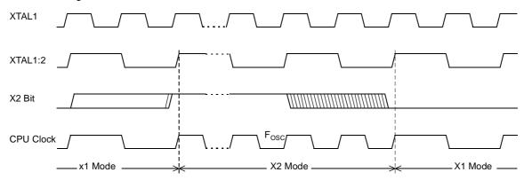
The X2 bit in the CKCON0 register (see Table 15) allows a switch from 12 clock periods per instruction to 6 clock periods and vice versa. At reset, the speed is set according to X2 bit of Hardware Security Byte (HSB). By default, Standard mode is active. Setting the X2 bit activates the X2 feature (X2 mode).
