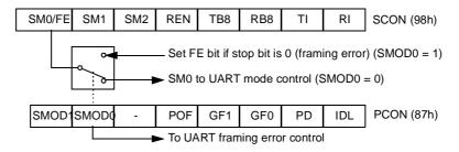
When this feature is enabled, the receiver checks each incoming data frame for a valid stop bit. An invalid stop bit may result from noise on the serial lines or from simultaneous transmission by two CPUs. If a valid stop bit is not found, the Framing Error bit (FE) in SCON register (See Table 33.) bit is set.
