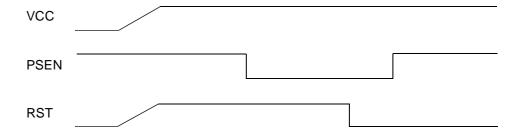
The on-chip bootloader boot process is shown in Figure 39.
