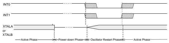
Exit from Power-down by reset redefines all the SFRs, exit from Power-down by external interrupt does no affect the SFRs.
