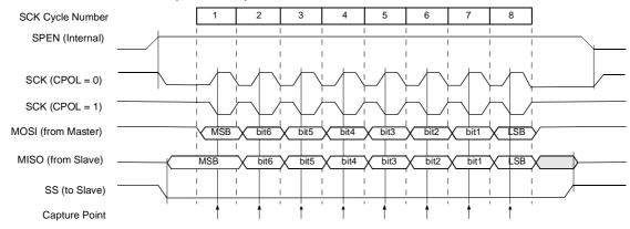
Figure 29. Data Transmission Format (CPHA = 1)
