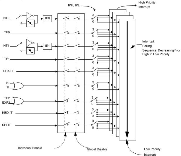
Each of the interrupt sources can be individually enabled or disabled by setting or clearing a bit in the Interrupt Enable register (Table 45 and Table 47). This register also contains a global disable bit, which must be cleared to disable all interrupts at once.
