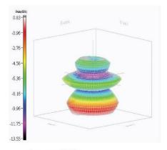
Frequency= 433 MHz Max gain = 0.83 dBi, at (150,330)
