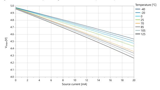
Figure 32-26. I/O Pin Output Voltage vs. Source Current (T = 25°C)
