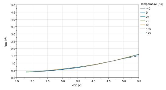
Figure 32-36. BOD Current vs. V<sub>DD</sub> (Sampled BOD at 1 kHz)
