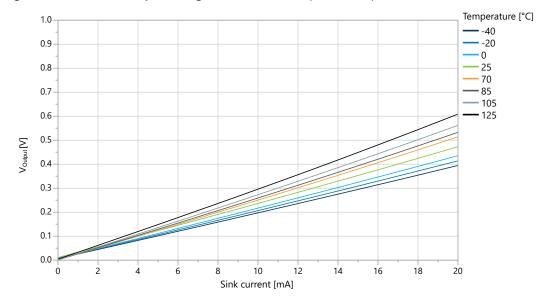
Figure 32-22. I/O Pin Output Voltage vs. Sink Current (T = 25°C)
