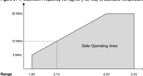
Figure 31-1. Maximum Frequency vs. V<sub>DD</sub> for [-40, 105]°C, Standard Temperature
