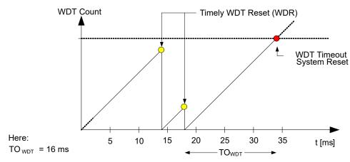
Normal mode is enabled as long as the WINDOW bit field in the Control A (WDT.CTRLA) register is 0x0.
