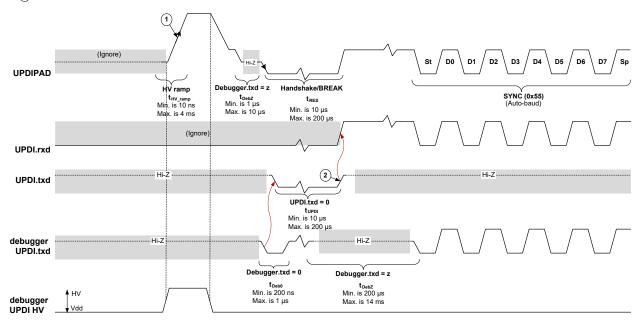
When enabled by an HV pulse, only a POR will disable the UPDI configuration on the RESET pin and restore the default setting. If issuing a UPDI Disable command through the UPDIDIS bit in UPDI.CTRLB, the UPDI will be reset, and the clock request will be canceled, but the RESET pin will remain in UPDI configuration.
