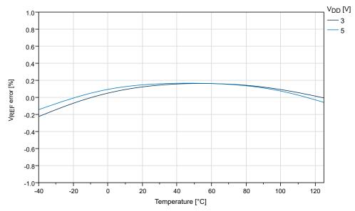
Figure 32-33. Internal 4.3V Reference vs. Temperature
