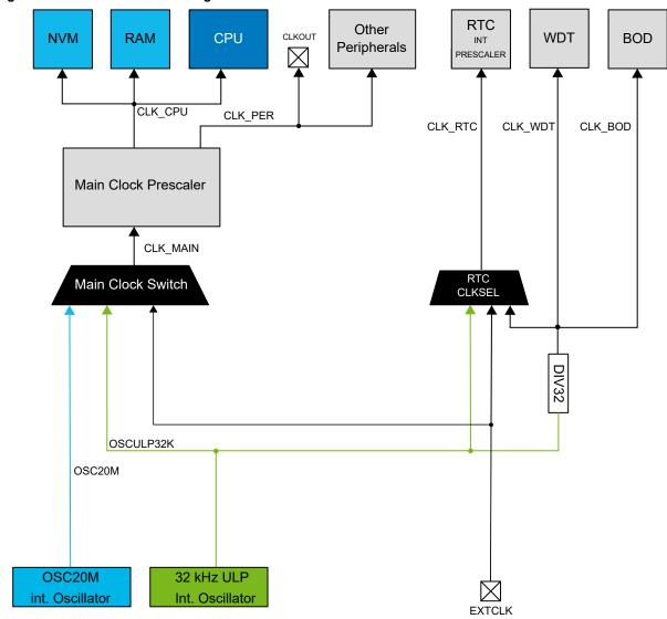
**Note:** The availability of the CLKOUT pin depends on the pin count of the device. See section 5. I/O Multiplexing and Considerations for an overview of which pins are available for each device represented in this data sheet.
