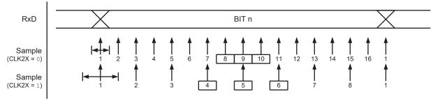
A majority voting technique is, like with clock recovery, used on the three center samples for deciding the logic level of the received bit. The process is repeated for each bit until a complete frame is received.
