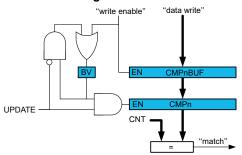
Both the TCAn.CMPn and TCAn.CMPnBUF registers are available as I/O registers. This allows the initialization and bypassing of the buffer register and the double-buffering function.
