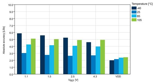
Figure 32-41. Absolute Accuracy vs.  $V_{REF}$  ( $V_{DD}$  = 5.0V,  $f_{ADC}$  = 115 ksps), REFSEL = Internal Reference
