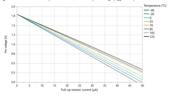
Figure 32-28. I/O Pin Pull-Up Resistor Current vs. Input Voltage ( $V_{DD} = 3.0V$ )
