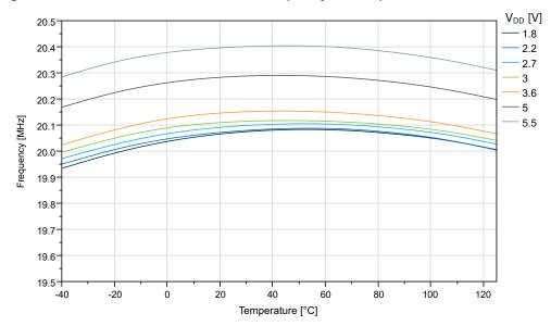
Figure 32-60. OSC20M Internal Oscillator: Frequency vs.  $V_{DD}$
