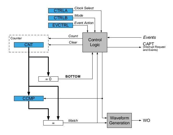
The timer/counter can be clocked from the Peripheral Clock (CLK\_PER) or a 16-bit Timer/Counter type A (CLK\_TCAn).
