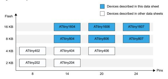
Devices with different Flash memory sizes typically also have different SRAM and EEPROM.
