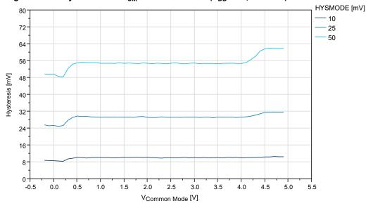
Figure 32-53. Offset vs.  $V_{CM}$  - 10 mV ( $V_{DD}$  = 5V)
