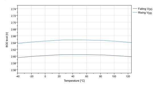
Figure 32-39. BOD Threshold vs. Temperature (Level 4.3V)
