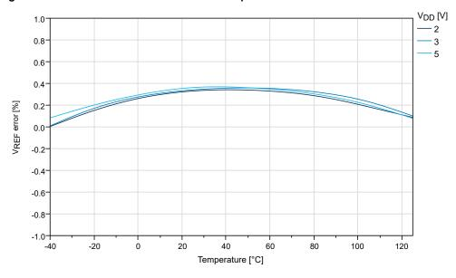
Figure 32-31. Internal 1.1V Reference vs. Temperature
