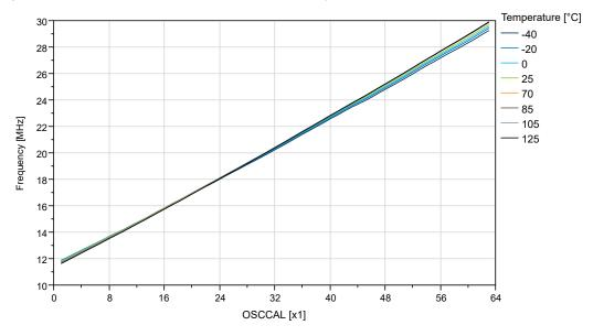
Figure 32-59. OSC20M Internal Oscillator: Frequency vs. Temperature
