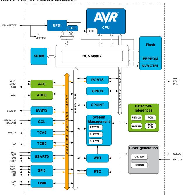
**Note:** The block diagram represents the largest device of the tinyAVR® 0-series, both in terms of pin count and Flash size. See sections 2.1 Configuration Summary and 5. I/O Multiplexing and Considerations for an overview of the features of the specific devices in this data sheet.
