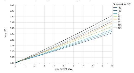
Figure 32-21. I/O Pin Output Voltage vs. Sink Current (V<sub>DD</sub> = 5.0V)
