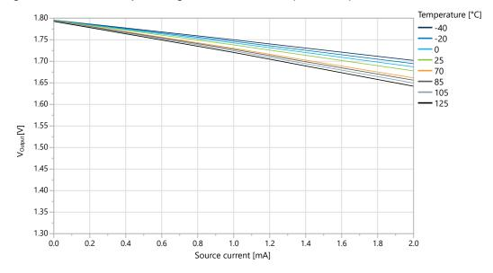
Figure 32-24. I/O Pin Output Voltage vs. Source Current (V<sub>DD</sub> = 3.0V)
