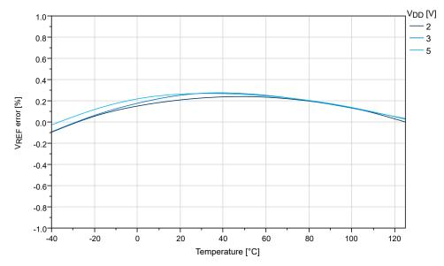
Figure 32-32. Internal 2.5V Reference vs. Temperature
