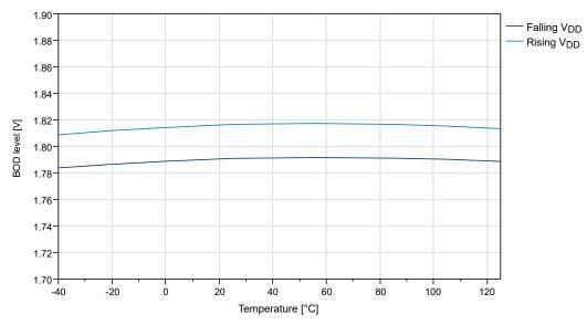
Figure 32-38. BOD Threshold vs. Temperature (Level 2.6V)
