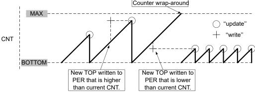
A counter wrap-around can occur in any mode of operation when counting up without buffering, as the TCAn.CNT and TCAn.PER registers are continuously compared. If a new TOP value is written to TCAn.PER that is lower than the current TCAn.CNT, the counter will wrap first, before a compare match occurs.
