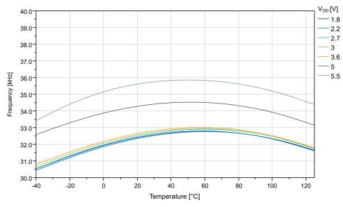
Figure 32-62. OSCULP32K Internal Oscillator Frequency vs. V<sub>DD</sub>
