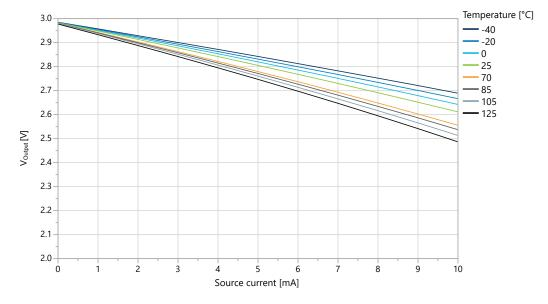
Figure 32-25. I/O Pin Output Voltage vs. Source Current (V<sub>DD</sub> = 5.0V)
