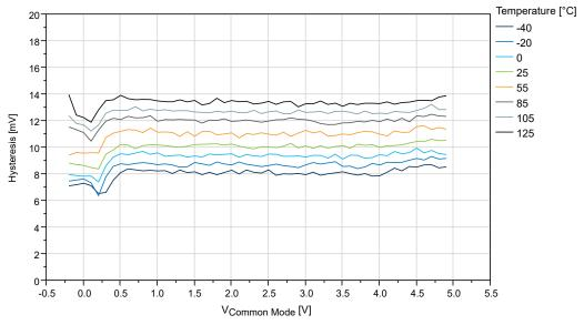
Figure 32-52. Hysteresis vs.  $V_{CM}$  - 10 mV to 50 mV ( $V_{DD}$  = 5V, T = 25°C)
