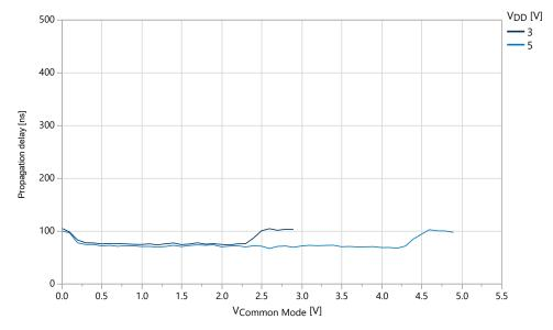
Figure 32-56. Propagation Delay vs.  $V_{CM}$  Rising Positive Input,  $V_{OD}$  = 30 mV (T = 25°C)
