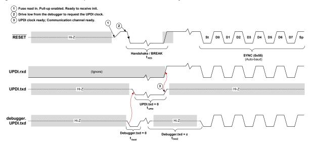
When the negative edge is detected, the UPDI clock starts. The UPDI will continue to drive the line low until the clock is stable and ready for the UPDI to use. The duration of t<sub>UPDI</sub> will vary, depending on the status of the oscillator when the UPDI is enabled. After this duration, the data line will be released by the UPDI and pulled high.
