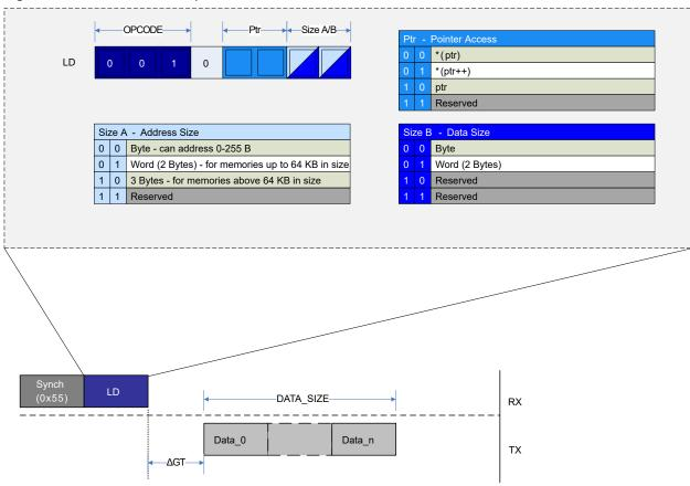
The figure above shows an example of a typical LD sequence, where the data are received after the Guard Time (GT) period. Loading data from the UPDI Pointer register follows the same transmission protocol.
