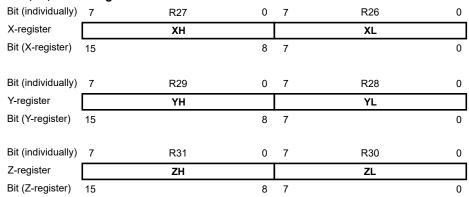
The lowest register address holds the Least Significant Byte (LSB), and the highest register address holds the Most Significant Byte (MSB). These address registers can function as fixed displacement, automatic increment, and automatic decrement, with different LD\*/ST\* instructions. See the *Instruction Set Summary* section for details.
