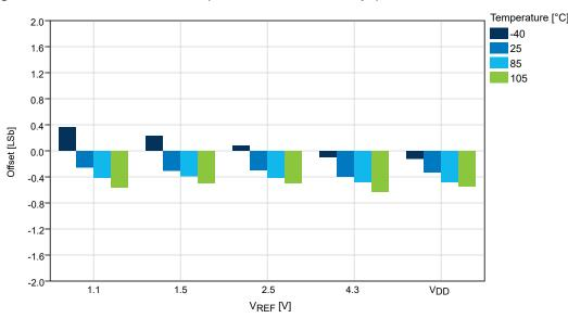
Figure 32-49. Offset Error vs. V<sub>REF</sub> (V<sub>DD</sub> = 5.0V, f<sub>ADC</sub> = 115 ksps), REFSEL = Internal Reference
