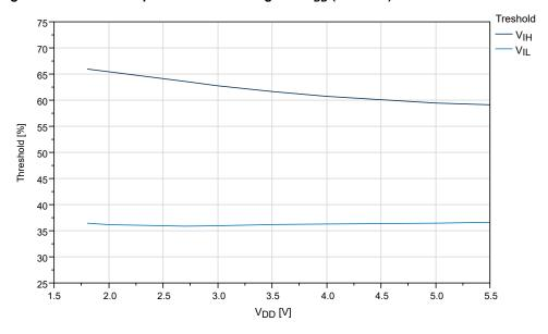
Figure 32-17. I/O Pin Input Threshold Voltage vs. V<sub>DD</sub> (V<sub>IH</sub>)
