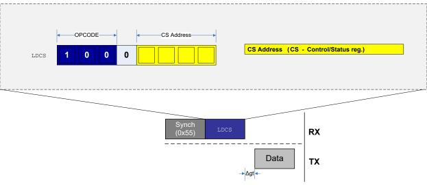
Figure 30-12 shows a typical example of LDCS data transmission. A data byte from the LDCS is transmitted from the UPDI after the guard time is completed.
