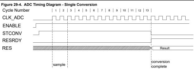
Both sampling time and sampling length can be adjusted using the Sample Delay (SAMPDLY) bit field in the Control D (ADCn.CTRLD) register and the Sample Length (SAMPLEN) bit field in the Sample Control (ADCn.SAMPCTRL) register. Both of these control the ADC sampling time in some CLK\_ADC cycles. This allows sampling of high-impedance sources without relaxing conversion speed. See the register description for further information. Total sampling time is given by:
