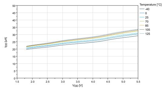
Figure 32-35. BOD Current vs. V<sub>DD</sub> (Sampled BOD at 125 Hz)
