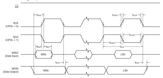
Figure 31-6. SPI - Timing Requirements in Client Mode
