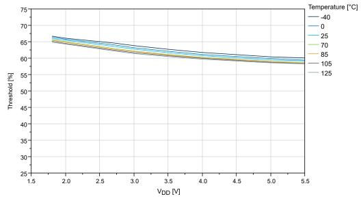
Figure 32-18. I/O Pin Input Threshold Voltage vs. V<sub>DD</sub> (V<sub>IL</sub>)
