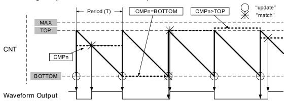
**Note:** The maximum duty-cycle of the waveform output is TOP/(TOP+1)
