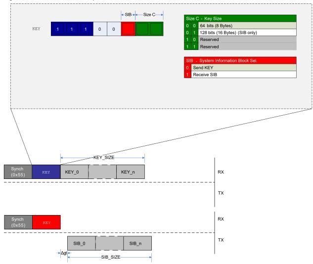
Figure 30-16 shows the transmission of a key and the reception of a SIB. In both cases, the Size C (SIZE\_C) field in the operand determines the number of frames being sent or received. There is no response after sending a KEY to the UPDI. When requesting the SIB, data will be transmitted from the UPDI according to the current guard time setting.
