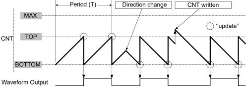
The following equation defines the waveform frequency ( $f_{FRO}$ ):
