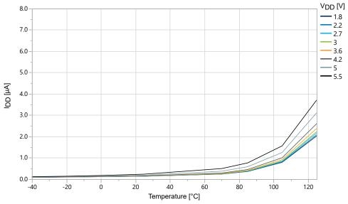
Figure 32-14. Power-Down Mode Supply Current vs. V<sub>DD</sub> (All Functions Disabled)
