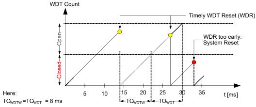
The Window mode is enabled by writing a non-zero value to the WINDOW bit field in the Control A (WDT.CTRLA) register, and disabled by writing it to 0x0.
