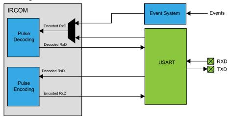
The USART is set in IRCOM mode by writing 0x02 to the CMODE bit field in the USARTn.CTRLC register. The data on the TXD/RXD pins are the inverted values of the transmitted/received infrared pulse. It is also possible to select an event channel from the Event System as an input for the IRCOM receiver. This enables the IRCOM to receive input from the I/O pins or sources other than the corresponding RXD pin, which will disable the RxD input from the USART pin.
