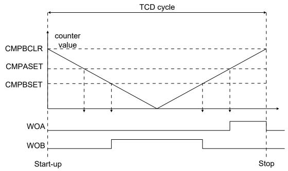
Figure 22-8. Dual Slope Mode Starting and Stopping
