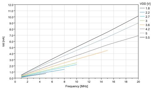
Figure 34-2. Active Supply Current vs. Frequency [0.1, 1.0]MHz at T=25°C
