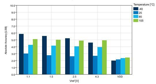
Figure 34-43. Absolute Accuracy vs.  $V_{ref}$  ( $V_{DD}$ =5.0V, 115ksps)
