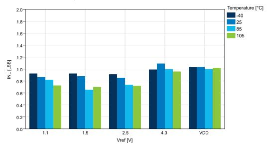
Figure 34-49. INL vs. V<sub>ref</sub> (V<sub>DD</sub>=5.0V, 115ksps)
