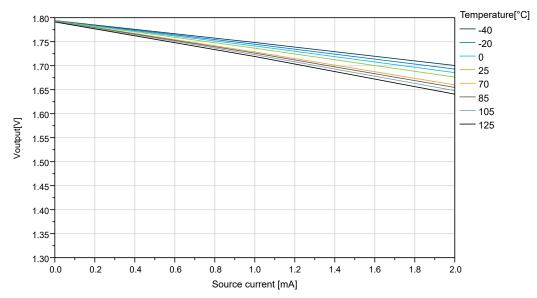
Figure 34-25. IO Pin Output Voltage vs. Source Current (V<sub>DD</sub>=1.8V)
