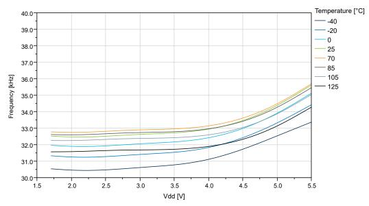
Figure 34-61. OSCULP32K Internal Oscillator Frequency vs. V<sub>DD</sub>
