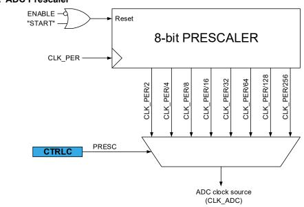
The ADC requires an input clock frequency between 50kHz and 1.5MHz for maximum resolution. If a lower resolution than 10 bits is selected, the input clock frequency to the ADC can be higher than 1.5MHz to get a higher sample rate.
