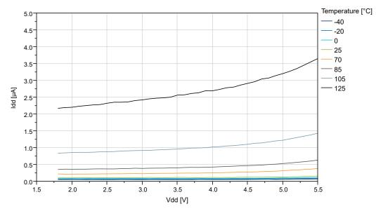
Figure 34-11. Power Down Mode Supply Current vs. V<sub>DD</sub> (all functions disabled)
