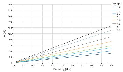
Figure 34-7. Idle Supply Current vs. Low Frequency (0.1-1.0MHz) at T=25°C
