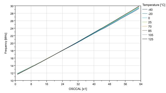
Figure 34-57. OSC20M internal Oscillator: Frequency vs. Calibration Value (V<sub>DD</sub>=3V)
