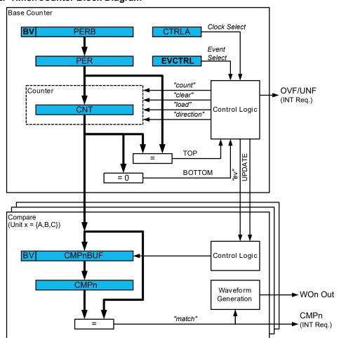
Figure 20-2. Timer/Counter Block Diagram
