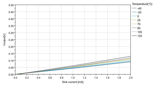
Figure 34-22. IO Pin Output Voltage vs. Sink Current (V<sub>DD</sub>=3.0V)
