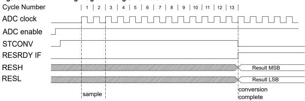
Both sampling time and sampling length can be adjusted using Sample Delay bit field in Control D (ADC.CTRLD) and sampling Sample Length bit field in the Sample Control register (ADC.SAMPCTRL). Both of these control the ADC sampling time in number of CLK\_ADC cycles. This allows sampling highimpedance sources without relaxing conversion speed. See register description for further information. Total sampling time is given by:
