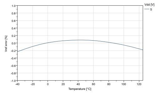
Figure 34-35. Internal 4.3V Reference vs. Temperature
