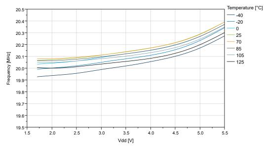
Figure 34-59. OSC20M Internal Oscillator: Frequency vs. V<sub>DD</sub>
