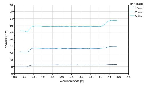
Figure 34-53. Hysteresis vs.  $V_{CM}$  - 10mV to 50mV ( $V_{DD}$ =5V, T=25°C)
