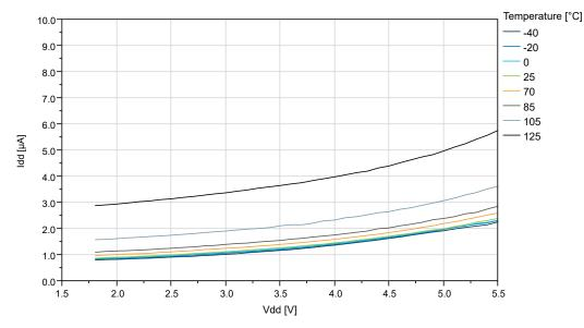
Figure 34-15. Standby Mode Supply Current vs. V<sub>DD</sub> (Sampled BOD running at 1kHz)
