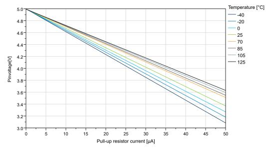
Figure 34-31. IO Pin Pull-Up Resistor Current vs. Input Voltage (V<sub>DD</sub>=5.0V)
