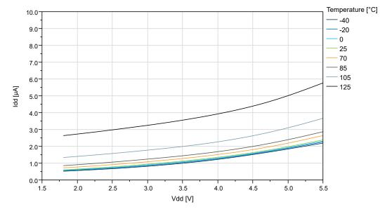
Figure 34-13. Standby Mode Supply Current vs. V<sub>DD</sub> (RTC running with internal OSCULP32K)
