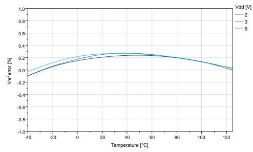
Figure 34-33. Internal 1.1V Reference vs. Temperature
