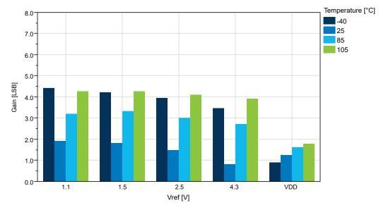
Figure 34-47. Gain Error vs.  $V_{ref}$  ( $V_{DD}$ =5.0V, 115ksps)
