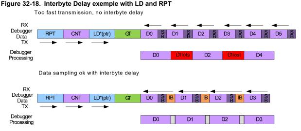
In Figure 32-18, GT denotes the Guard Time insertion, SB are stop bits and IB is the inserted interbyte delay. The rest of the frames are data and instructions.
