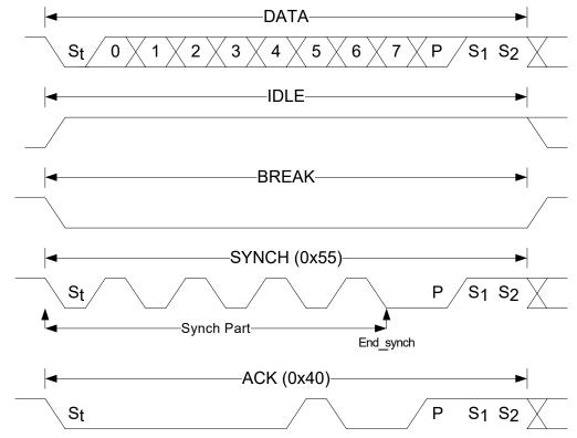
DataConsist of 1 start bit (always low), 8 data bits, 1 parity bit (even parity) and two stop bitsFrame(always high). If the start bit, parity bit or stop bits have an incorrect value, an error will be<br/>detected and signalized by the UPDI. The parity bit check in the UPDI can be disabled by<br/>writing the PARD bit in UPDI.CTRLA, in which case the parity generation from the debugger<br/>can be ignored.
