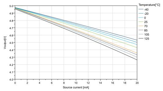
Figure 34-27. IO Pin Output Voltage vs. Source Current (V<sub>DD</sub>=5.0V)
