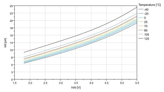
Figure 34-5. Active Supply Current vs. V<sub>DD</sub> (f=32KHz OSCULP32K)
