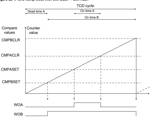
Figure 22-4. One Ramp Mode with CMPBSET < CMPASET
