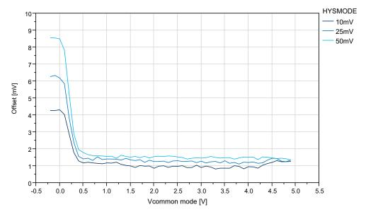
Figure 34-55. Offset vs.  $V_{CM}$  - 10mV to 50mV (V\_{DD}=5V, T=25°C)
