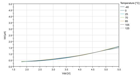
Figure 34-37. BOD Current vs. V<sub>DD</sub> (Sampled BOD at 125Hz)
