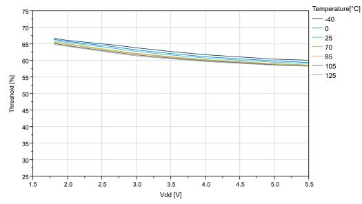
Figure 34-19. IO Pin Input Threshold Voltage vs. V<sub>DD</sub> (V<sub>IH</sub>)
