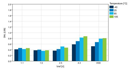
Figure 34-45. DNL vs. V<sub>ref</sub> (V<sub>DD</sub>=5.0V, 115ksps)
