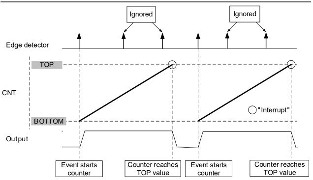
If the ASYNC bit in TCB.CTRLB is '0', the event pulse needs to be longer than one system clock cycle in order to guarantee edge detection.
