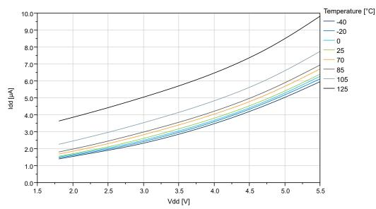
Figure 34-9. Idle Supply Current vs. V<sub>DD</sub> (f=32KHz OSCULP32K)
