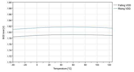
Figure 34-40. BOD Threshold vs. Temperature (Level 2.6V)
