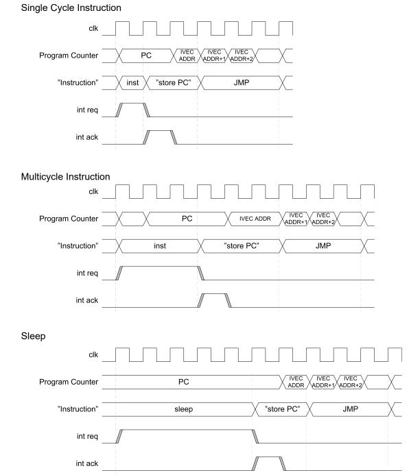
If an interrupt occurs when the device is in sleep mode, the interrupt execution response time is increased by five clock cycles. In addition, the response time is increased by the start-up time from the selected sleep mode.
