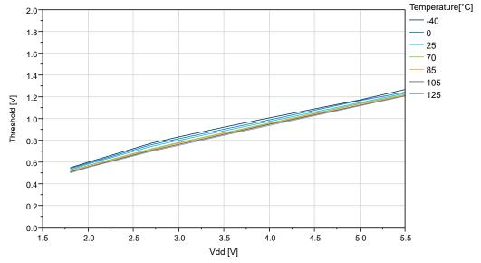
Figure 34-18. IO Pin Input Threshold Voltage vs. V<sub>DD</sub> (T=25°C)
