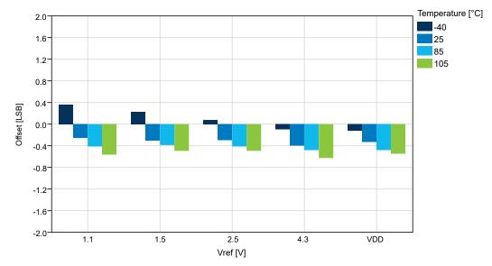
Figure 34-51. Offset Error vs. V<sub>ref</sub> (V<sub>DD</sub>=5.0V, 115ksps)
