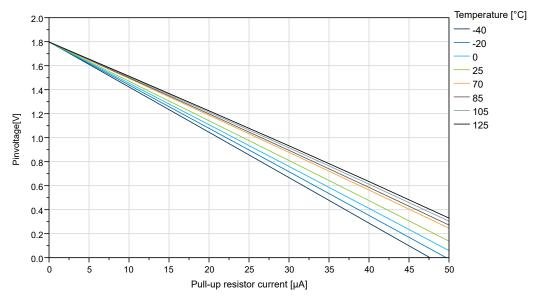
Figure 34-30. IO Pin Pull-Up Resistor Current vs. Input Voltage (V<sub>DD</sub>=3.0V)
