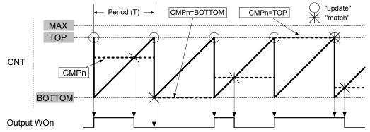
The TCA.PER register defines the PWM resolution. The minimum resolution is 2 bits (TCA.PER=0x0003), and the maximum resolution is 16 bits (TCA.PER=MAX).
