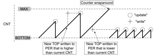
A counter wraparound can occur in any mode of operation when up-counting without buffering. This is due to the fact that the registers TCA.CNT and TCA.PER are continuously compared: if a new TOP value is written to TCA.PER that is lower than current TCA.CNT, the counter will wrap first before a compare match happened.
