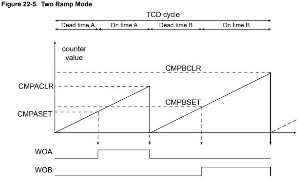
In the figure above, *CMPASET < CMPACLR and CMPBSET < CMPBCLR*. This causes the outputs to go high. There are no restrictions on the CMPASET/CLR compared to the CMPBSET/CLR values.
