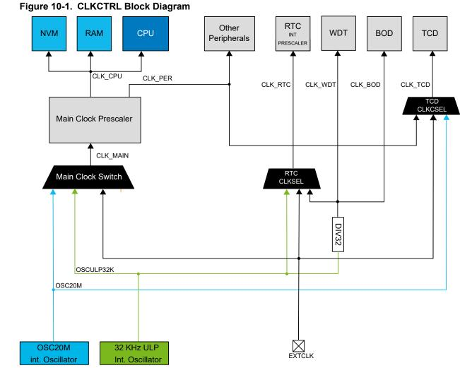
The clock system consists of the Main Clock and other asynchronous clocks:
