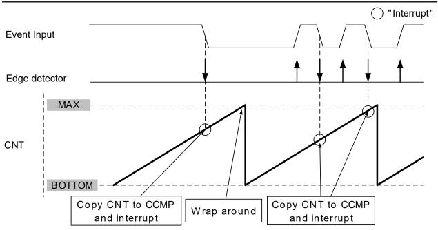
It is recommended to write zero to the TCB.CNT register when entering this mode from any other mode.
