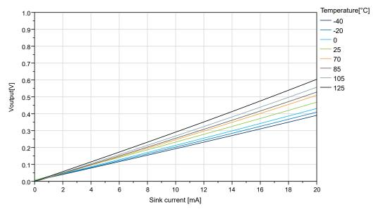
Figure 34-23. IO Pin Output Voltage vs. Sink Current (V<sub>DD</sub>=5.0V)
