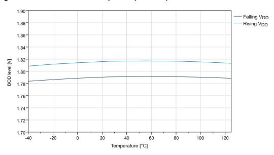
Figure 36-39. BOD Threshold vs. Temperature (Level 2.6V)
