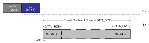
For LD, data will come out continuously after the LD instruction. Note the guard time on the first data block.
