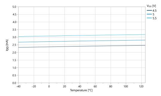
Figure 36-9. Idle Supply Current vs. V<sub>DD</sub> (f = 32.768 kHz OSCULP32K)
