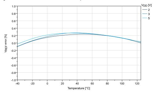
Figure 36-33. Internal 2.5V Reference vs. Temperature
