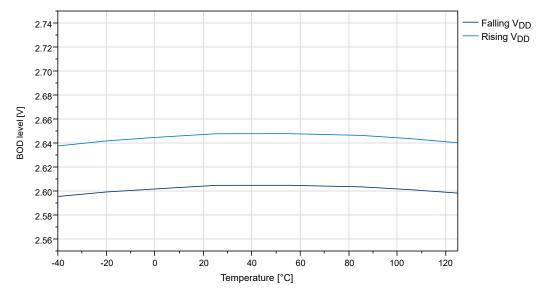
Figure 36-40. BOD Threshold vs. Temperature (Level 4.3V)
