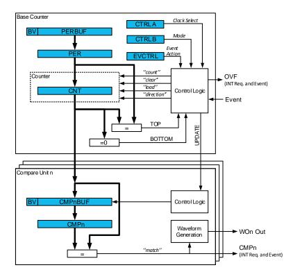
The Counter (TCAn.CNT) register, Period and Compare (TCAn.PER and TCAn.CMPn) registers, and their corresponding buffer registers (TCAn.PERBUF and TCAn.CMPnBUF) are 16-bit registers. All buffer registers have a Buffer Valid (BV) flag that indicates when the buffer contains a new value.
