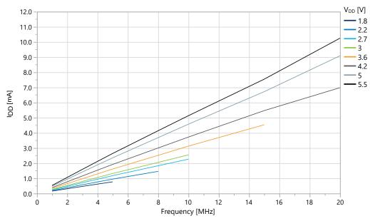
Figure 36-2. Active Supply Current vs. Frequency [0.1, 1.0] MHz at T = 25°C (EXTCLK)
