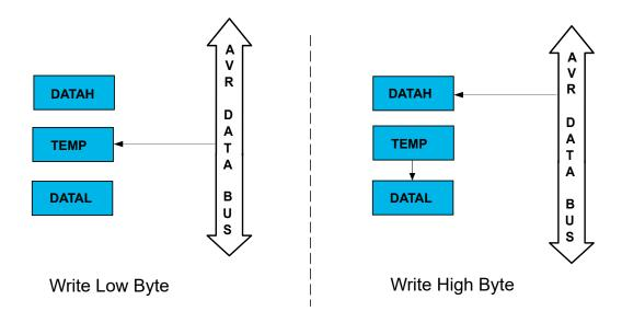
For a 16-bit write operation, the low byte register (e.g. DATAL) of the 16-bit register must be written before the high byte register (e.g. DATAH). Writing the low byte register will result in a write to the temporary (TEMP) register instead of the low byte register, as shown in the left side of Figure 8-6. When the high byte register of the 16-bit register is written, TEMP will be copied into the low byte of the 16-bit register in the same clock cycle, as shown in the right side of Figure 8-6.
