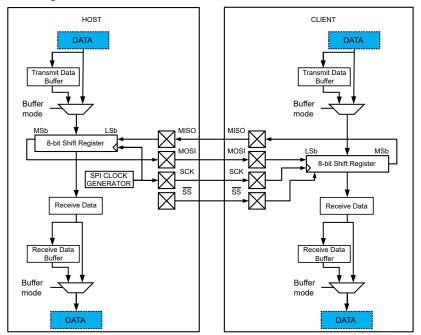
The SPI is built around an 8-bit shift register that will shift data out and in at the same time. The Transmit Data register and the Receive Data register are not physical registers but are mapped to other registers when written or
