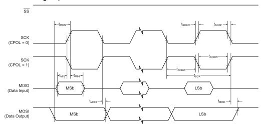
Figure 35-6. SPI - Timing Requirements in Client Mode
