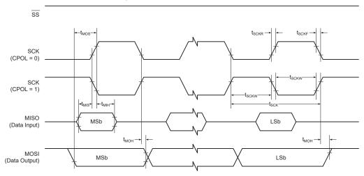
Table 35-18. USART in SPI Host Mode - Timing Characteristics
