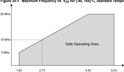
Figure 35-1. Maximum Frequency vs. V<sub>DD</sub> for [-40, 105]°C, Standard Temperature Range
