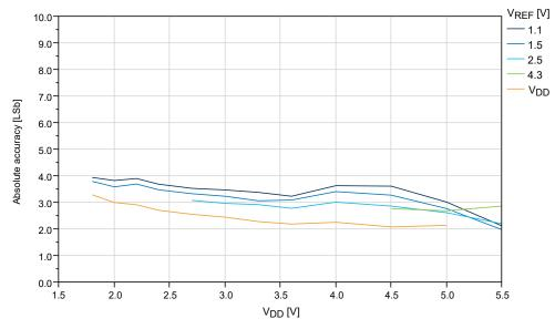
Figure 36-42. Absolute Accuracy vs. V<sub>REF</sub> (V<sub>DD</sub> = 5.0V, f<sub>ADC</sub> = 115 ksps), REFSEL = Internal Reference
