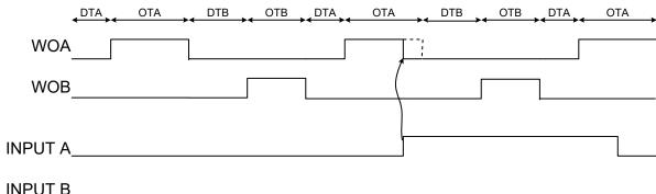
If Input mode 9 is used on input B and a positive edge on the input event occurs while in on time B, the output will be OFF for the rest of the on time.
