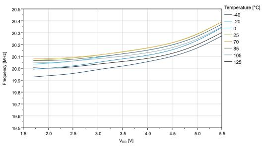
Figure 36-63. OSC20M Internal Oscillator: Frequency vs. V<sub>DD</sub>
