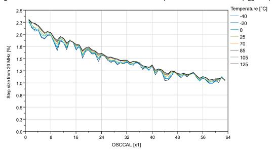
Figure 36-61. OSC20M Internal Oscillator: Frequency vs. Calibration Value ( $V_{DD} = 3V$ )
