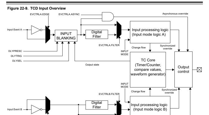
There is a delay of two/three clock cycles on the TCD synchronizer clock between receiving the input event, processing it, and overriding the outputs. If using the asynchronous event detection, the outputs will override instantly outside the input processing.
