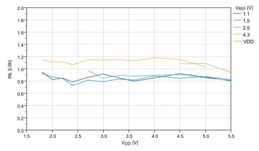
Figure 36-48. INL vs.  $V_{REF}$  ( $V_{DD}$  = 5.0V,  $f_{ADC}$  = 115 ksps), REFSEL = Internal Reference
