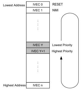
Here, value Y has been written to CPUINT.LVL0PRI, so that interrupt vector Y+1 has the highest priority. Note that, in this case, the priorities will wrap so that the lowest address no longer has the highest priority. This does not include RESET and NMI, which will always have the highest priority.
