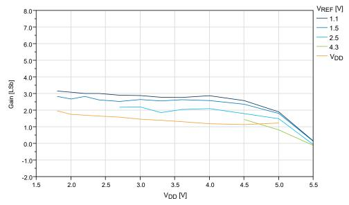
Figure 36-46. Gain Error vs.  $V_{REF}$  ( $V_{DD}$  = 5.0V,  $f_{ADC}$  = 115 ksps), REFSEL = Internal Reference
