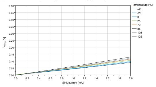
Figure 36-21. I/O Pin Output Voltage vs. Sink Current (V<sub>DD</sub> = 3.0V)
