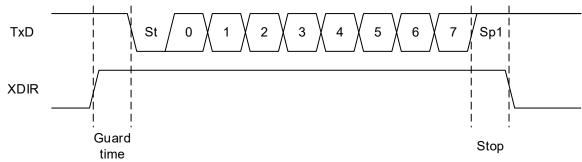
Writing RS485[1] to '1' enables the RS-485 mode, which automatically sets the TXD pin to output one clock cycle before starting transmission and sets it back to input when the transmission is complete.
