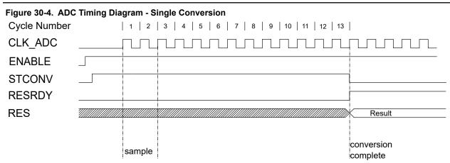
Both sampling time and sampling length can be adjusted using the Sample Delay bit field in the Control D (ADCn.CTRLD) register and the Sample Length bit field in the Sample Control (ADCn.SAMPCTRL) register. Both of these control the ADC sampling time in some CLK\_ADC cycles. This allows sampling of high-impedance sources without relaxing conversion speed. See the register description for further information. Total sampling time is given by:
