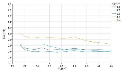
Figure 36-44. DNL vs.  $V_{REF}$  ( $V_{DD}$  = 5.0V,  $f_{ADC}$  = 115 ksps), REFSEL = Internal Reference
