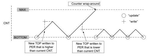
**With Buffering:** When double-buffering is used, the buffer can be written at any time and still maintain the correct operation. The TCAn.PER is always updated on the UPDATE condition, as shown for dual-slope operation in the figure below. This prevents wrap-around and the generation of odd waveforms.
