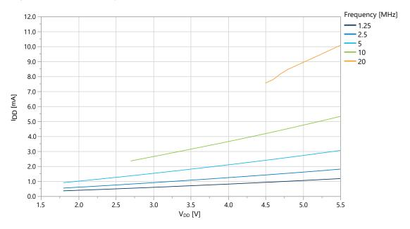
Figure 36-5. Active Supply Current vs. V<sub>DD</sub> (f = 32.768 kHz OSCULP32K)
