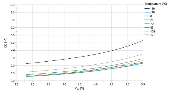
Figure 36-12. Standby Mode Supply Current vs. V<sub>DD</sub> (Sampled BOD Running at 125 Hz)
