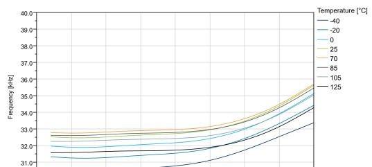
Figure 36-65. OSCULP32K Internal Oscillator Frequency vs. V<sub>DD</sub>
