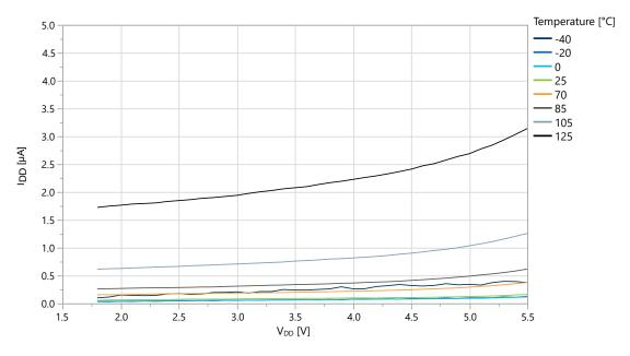
Figure 36-15. Power-Down Mode Supply Current vs. V<sub>DD</sub> (All Functions Disabled)
