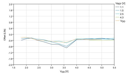
Figure 36-50. Offset Error vs.  $V_{REF}$  ( $V_{DD}$  = 5.0V,  $f_{ADC}$  = 115 ksps), REFSEL = Internal Reference
