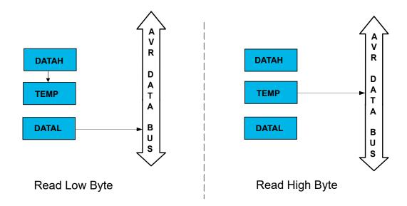
For a 16-bit read operation, the low byte register (e.g. DATAL) of the 16-bit register must be read before the high byte register (e.g. DATAH). When the low byte register is read, the high byte register of the 16-bit register is copied into the temporary (TEMP) register in the same clock cycle, as show in the left side of Figure 8-7. Reading the high byte register will result in a read from TEMP instead of the high byte register, as shown in right side of Figure 8-7.
