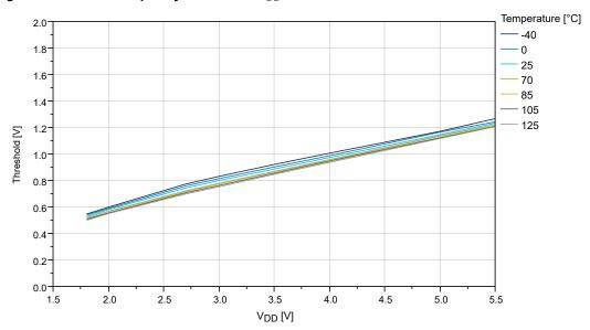
Figure 36-17. I/O Pin Input Threshold Voltage vs.  $V_{DD}$  (T = 25°C)
