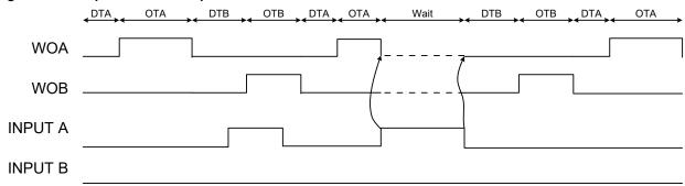
If Input mode 1 is used on input B, an event will only have an effect if the TCD is in dead time B or on time B, and it will only affect the WOB output. When the event is done, the TCD counter starts at dead time A.
