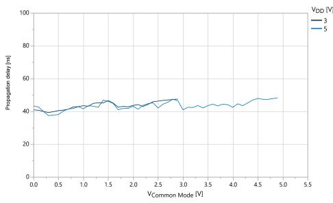
Figure 36-59. Propagation Delay vs.  $V_{CM}$  LPMODE Disabled, Rising Positive Input,  $V_{OD}$  = 30 mV (T = 25°C)
