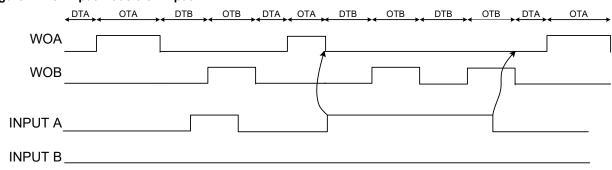
If Input mode 3 is used on input B, an event will only have an effect if the TCD is in dead time B or on time B.
