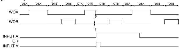
If Input mode 8 is used on input B and a positive edge on the input event occurs while in on time B, the TCD counter jumps to dead time A.
