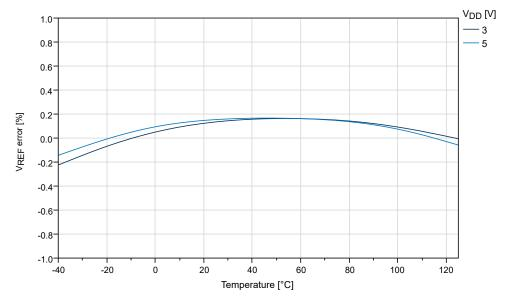
Figure 36-34. Internal 4.3V Reference vs. Temperature
