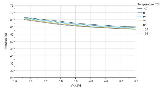
Figure 36-19. I/O Pin Input Threshold Voltage vs.  $V_{DD} \left( V_{IL} \right)$
