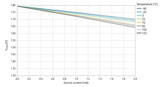
Figure 36-25. I/O Pin Output Voltage vs. Source Current (V<sub>DD</sub> = 3.0V)
