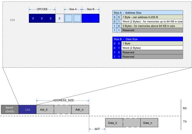
When the instruction is decoded, and the address byte(s) are received as dictated by the decoded instruction, the DL layer will synchronize all required information to the ACC layer, which will handle the bus request and synchronize data buffered from the bus back again to the DL layer. This will create a synchronization delay that must be taken into consideration upon receiving the data from the UPDI.
