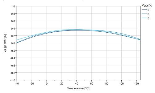
Figure 36-32. Internal 1.1V Reference vs. Temperature
