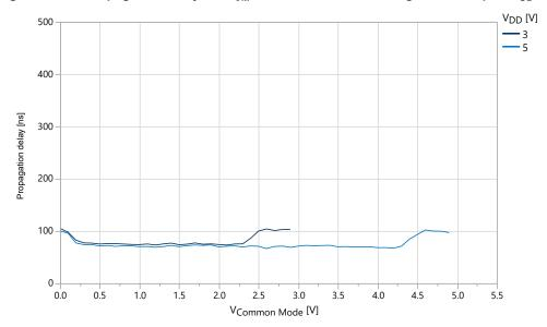
Figure 36-57. Propagation Delay vs.  $V_{CM}$  LPMODE Enabled, Rising Positive Input,  $V_{OD}$  = 30 mV (T = 25°C)
