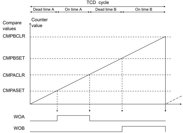
In the figure above, CMPASET < CMPACLR < CMPBSET < CMPBCLR. In One Ramp mode, this is required to avoid overlapping outputs during the on time. The figure below is an example where CMPBSET < CMPASET < CMPACLR < CMPBCLR, which has overlapping outputs during the on time.
