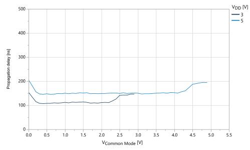
Figure 36-58. Propagation Delay vs.  $V_{CM}$  LPMODE Disabled, Falling Positive Input,  $V_{OD}$  = 30 mV (T = 25°C)
