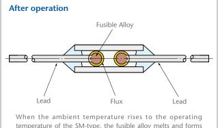
temperature of the SM-type, the fusible alloy melts and forms a drop around the end of each lead due to the surface tension and the special flux coating. Without a direct contact between the leads, the electrical circuit is opened.
