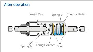
When the ambient temperature rises to the operating temperature of the SF-type, heat is transferred through the metal case and melts the thermal pellet. Springs A and B then stretch and the sliding contact moves away from lead A, thereby opening the electrical circuit.
