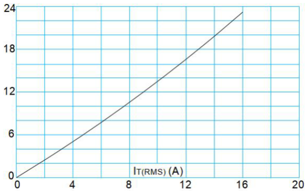
FIG.1: Maximum power dissipation versus RMS on-state current
