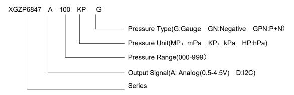
Note: 5Vdc as default power voltage, add 33(or 30) behind model signify 3.3V(or 3.0V) power supply, e.g. XGZP6847A040KPG33(or XGZP6847A040KPG30).
