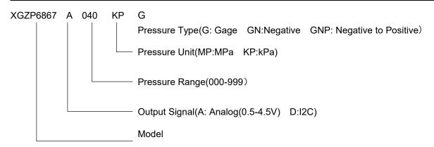
Note: 5Vdc as default power voltage, add 33(or 30) behind model signify 3.3V(or 3.0V) power supply, e.g. XGZP6867A040KPG33(or XGZP6867A040KPG30).
