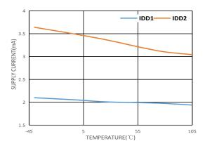
Figure 3. Unloaded Supply Current vs. Temperature
