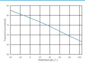
Figure 4. Transmit Current vs. Temperature, VDD1=5V, VDD2=5V
