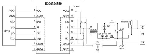
Figure 14. Port protection circuit for harsh environments
