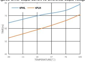
Figure 8. Receiver Progation Delay vs. Temperature
