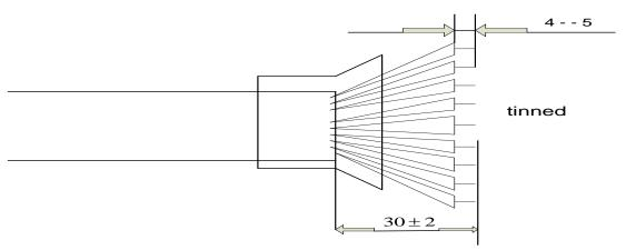
Figure 5.2 USB-RS422-WE Mechanical Details (dimensions in mm)
