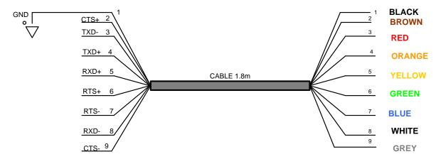
Figure 5.1 USB-RS422-WE Connections
