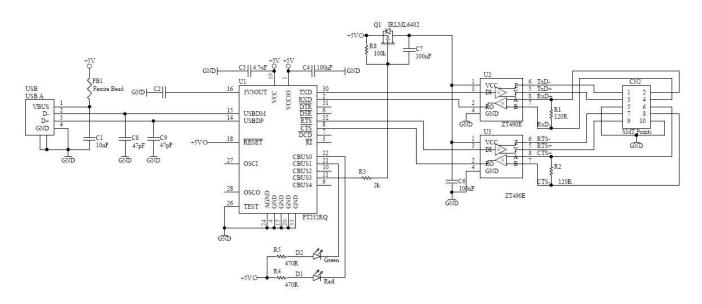
Figure 7.1 Schematic for USB-RS422 Converter Cable
