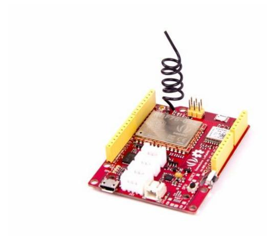
LoRaWAN Class A/C Ultra long range of communication GPS communication Ultra low power consumption Arduino programming (based on Arduino Zero bootloader) Embeded with lithim battery management chip 4 Grove connectors onboard
