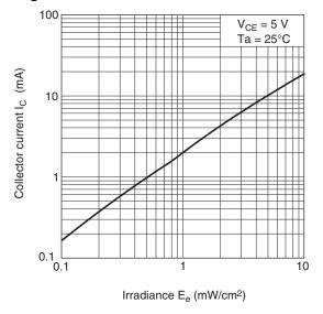
Fig. 5 Collector Current vs.
