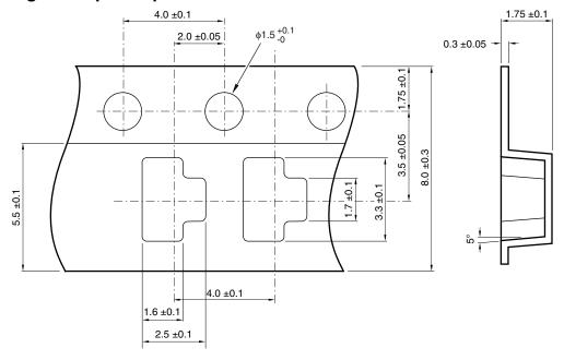
Fig. 12 Reel Shape and Dimension
