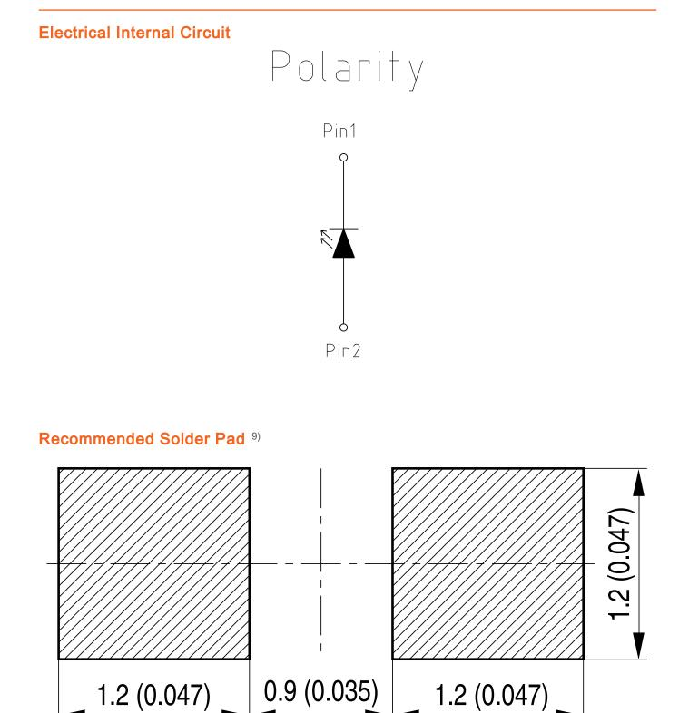
For superior solder joint connectivity results we recommend soldering under standard nitrogen atmosphere. Package not
