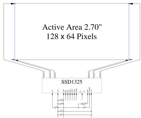
MCU Interface Selection: BS1 and BS2 Pins connected to MCU interface: CS#, RES#, D/C#, R/W#, E/RD#, and D0~D7
