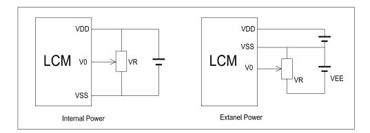
V<sub>DD-</sub>V<sub>0</sub>: LCD Driving voltage VR: 10k~20k
