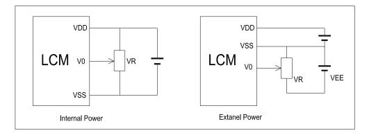
$V_{DD-}V_0$ : LCD Driving voltage VR: 10k~20k
