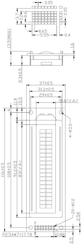
Display Type: STN-Blue/Negative/Transmissive/6:00 Visual Angle 1). Driver Method: 1/16duty, 1/5bias, VDD5.0V VLCD4.3V 2). Display Type: STN-Blue/Negative/Transmissive/6:00 Vi 3). Operating Temp: -20C~70°C/Storage Temp: -30°C~80° 4). Backlight Type: Edge/White 5). Driver: ST7066U/4bit or 8bit MPU 6). RoHS Compliant
