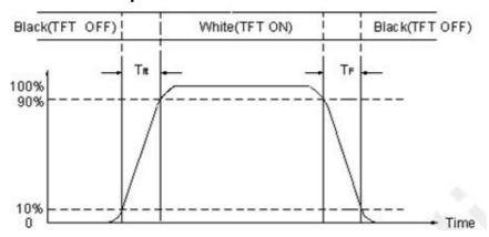
Note (4) Definition of optical measurement setup
