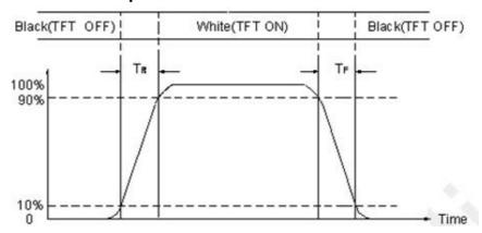
Note (4) Definition of optical measurement setup
