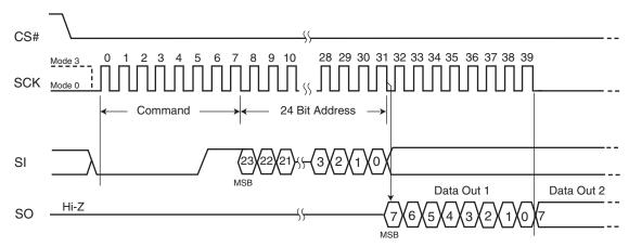
Figure 10. Read Data Bytes (READ) Command Sequence
