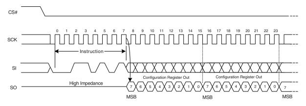
Figure 23. Read Configuration Register (RCR) Instruction Sequence
