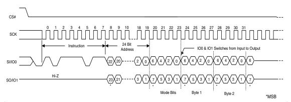
Figure 14. DUAL I/O High Performance Read Instruction Sequence
