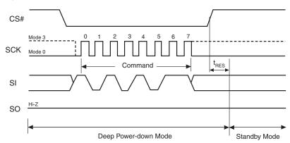
Figure 32. Release from Deep Power-Down (RES) Command Sequence
