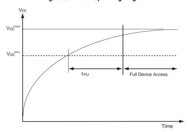
Figure 39. Power-Up Timing Diagram
