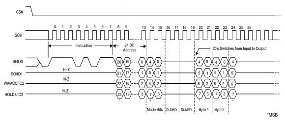
Figure 16. QUAD I/O High Performance Instruction Sequence
