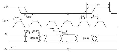
Figure 46. SPI Mode 0 (0,0) Output Timing
