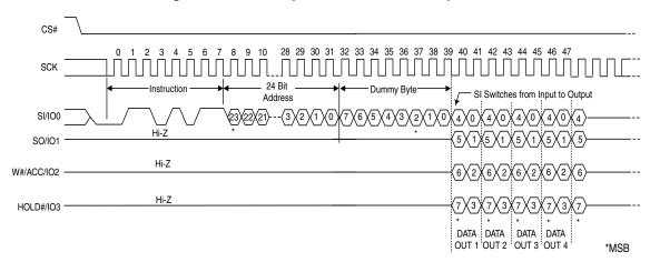
Figure 13. Quad Output Read Instruction Sequence
