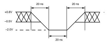
Figure 43. Maximum Positive Overshoot Waveform
