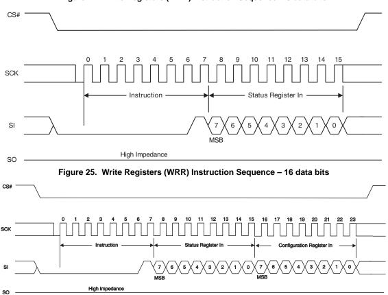
Figure 24. Write Registers (WRR) Instruction Sequence - 8 data bits
