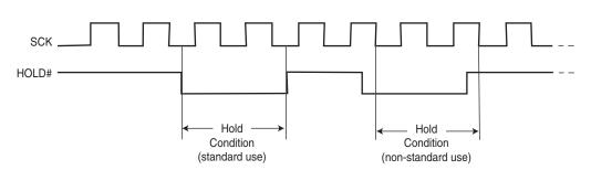
Figure 9. Hold Mode Operation
