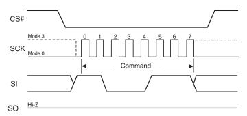
Figure 30. Bulk Erase (BE) Command Sequence
