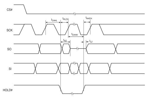
Figure 48. Write Protect Setup and Hold Timing during WRR when SRWD = 1
