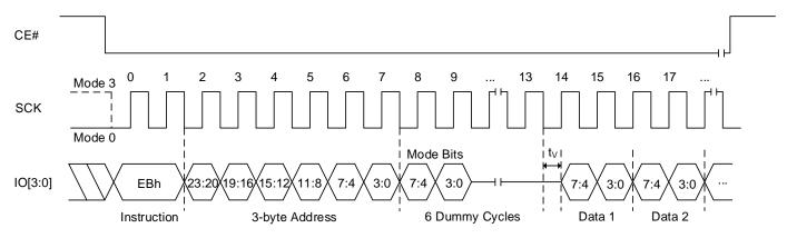
Note: Number of dummy cycles depends on Read Parameter setting. Detailed information in Table 6.10 Read Dummy Cycles.
