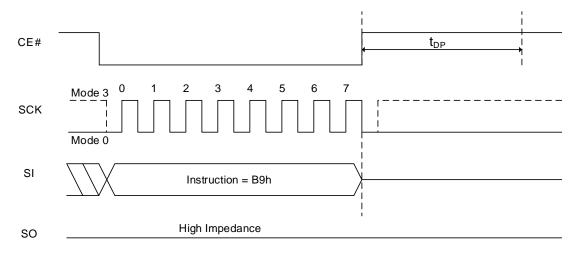
Figure 8.37 Enter Deep Power Down Mode QPI Sequence
