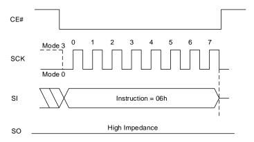
Figure 8.23 Write Enable QPI Sequence
