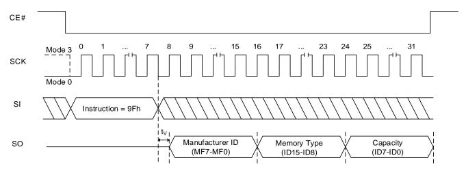
Figure 8.45 RDJDID and RDJDIDQ (Read JEDEC ID) Sequence in QPI Mode
