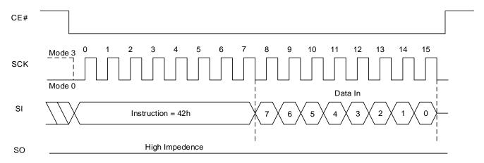
Figure 8.33 Write Function Register QPI Sequence
