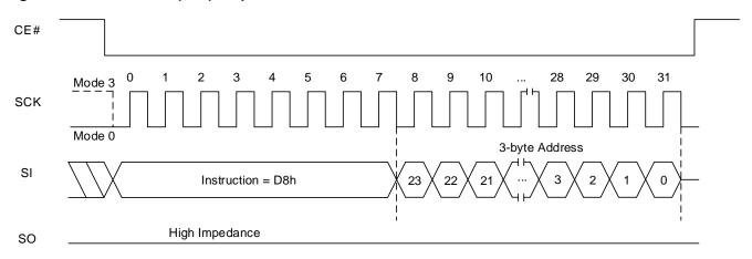
Figure 8.17 Block Erase (64K) QPI Sequence
