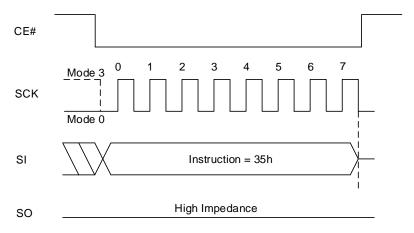
Figure 8.35 Exit Quad Peripheral Interface (QPI) Mode Sequence
