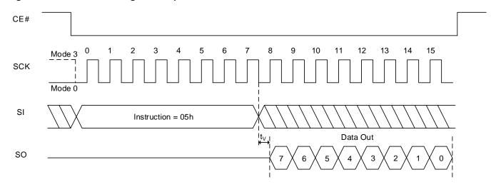
Figure 8.27 Read Status Register QPI Sequence
