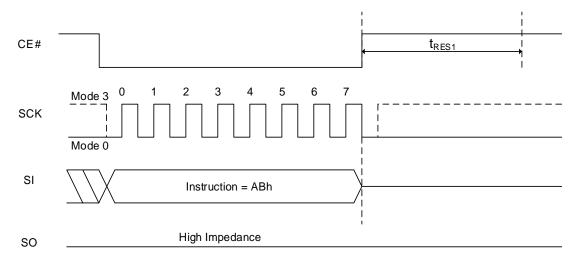
Figure 8.39 Release Power Down QPI Sequence
