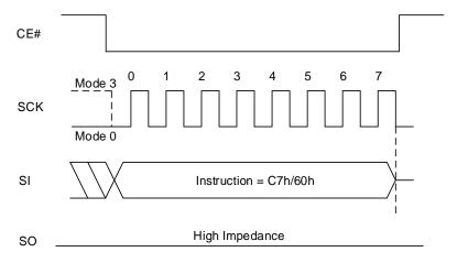
Figure 8.21 Chip Erase QPI Sequence
