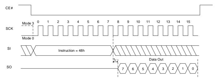
Figure 8.31 Read Function Register QPI Sequence
