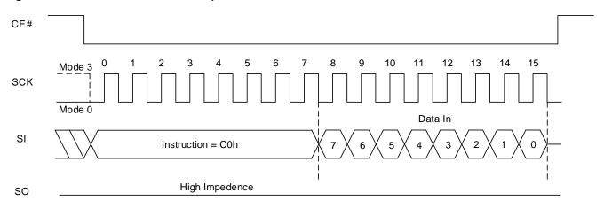
Figure 8.41 Set Read Parameters QPI Sequence
