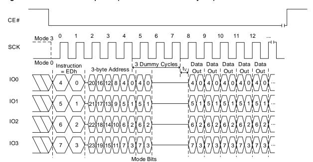
Figure 8.61 FRQDTR QPI Sequence (with command decode cycles)
