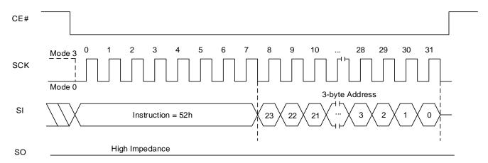
Figure 8.19 Block Erase (32K) QPI Sequence
