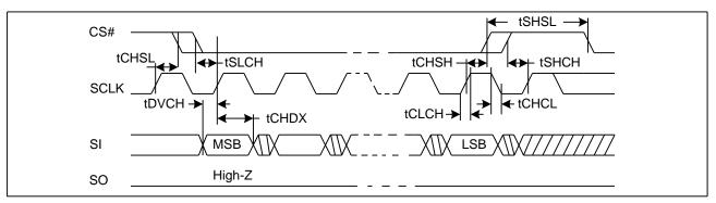
Figure41. Output Timing
