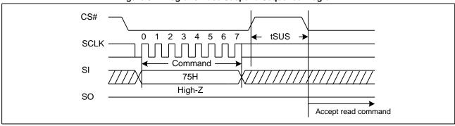
Figure 31. Program/Erase Suspend Sequence Diagram
