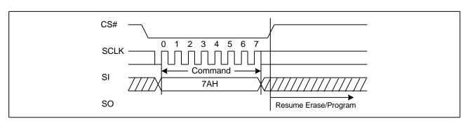
Figure 32. Program/Erase Resume Sequence Diagram
