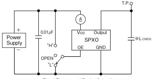
**%L-cmos: Total Fixture and Probe Capacitance**
