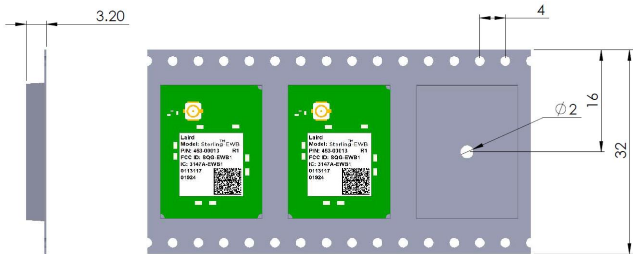
Figure 14: U.FL and chip antenna modules tape and reel specification (full reel contains 1000 modules)
