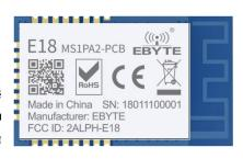
E18-MS1PA2-PCB adopts the original CC2530 RF chip of TI, the chip is integrated with 8051 MCU and wireless transceiver, and built-in PA+LNA, greatly expanding communication distance and improving communication stability. The module is applicable for ZigBee design and 2.4GHz IEEE 802.15.4 protocol.
