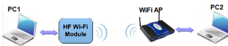
Figure 56. STA Interface Debug Connection
